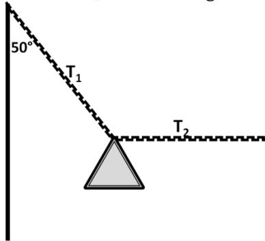
68. A body weight  $W$  is suspended from a frame as shown in the figure. If the magnitude of the tension of the rope  $T$  is 500 N and the angle is  $35^\circ$  to the horizontal. Determine the magnitude of the weight  $W$  and the thrust  $F$  of the bar.
